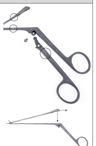
2. Lower the slider (5) onto the shaft. The slider (5) must be pulled back in the direction of the ring handle so that the mouth is opened to the maximum. Only in this way can the guide pins of the slider (6) be inserted into the guide rail of the shaft at the correct position.
