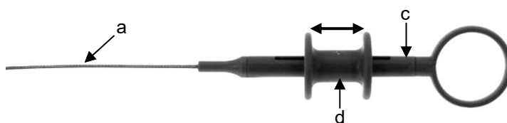
Fig. 1b: Pull roller handle of the myocardial biptome, proximal end
