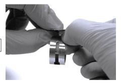
2. Place the guide tabs (1) over the insertion opening (2) and insert the guide tabs (1). Then release the pressure slightly and allow the guide tabs (1) to slide along the guide bar (3).
