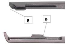
a) Place the slider with the spring (pos. 6) on the milled groove (pos. 7) in the punch body, and the front guide of the slider (pos. 8) on the guiding rail (pos. 9) of the punch body at the same time.
