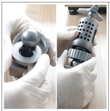
Slide the union nut over the ball, slide the washer with its recess around the ball neck so that it lies on the inner base of the union nut. The small bevel of the washer points towards the ball. Then screw the 3-part assembly with the union nut onto the clamping cylinder.
